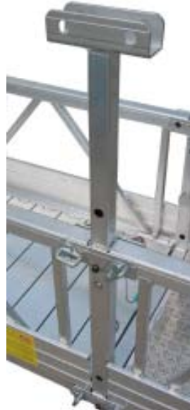
14. Install the locking brackets to prevent the custom decks from lifting up while suspended.
