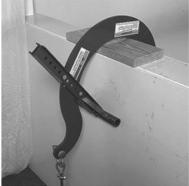
Similar to the Tank Top Roller, Ring Girder Rollers are used where a steel ring girder is located around a storage tank perimeter. Roller travels on rim of girder. It should be used in conjunction with hanging rope and tie back.
