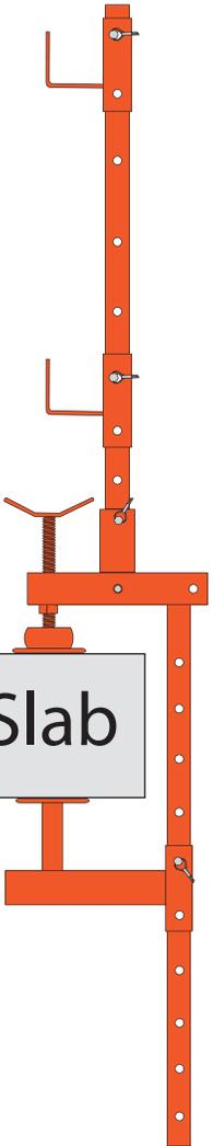
Base clamp swivels to adjust from a slab to a parapet in seconds!
