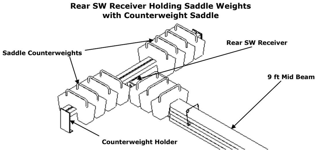
Flame cut weights are used with a LH Rear Receiver (WSOR344), use a Longhorn Bar. Thirty inch (WSOR43) and forty-two inch (WSOR70) Longhorn Bars are available. You attach the LH Rear Receiver to the Mid Beam (WSOR318) as shown below. Take care to lock all snap lock pins. If your weight system does not fall into either of these two categories, contact Winsafe for a custom weight holder system.
