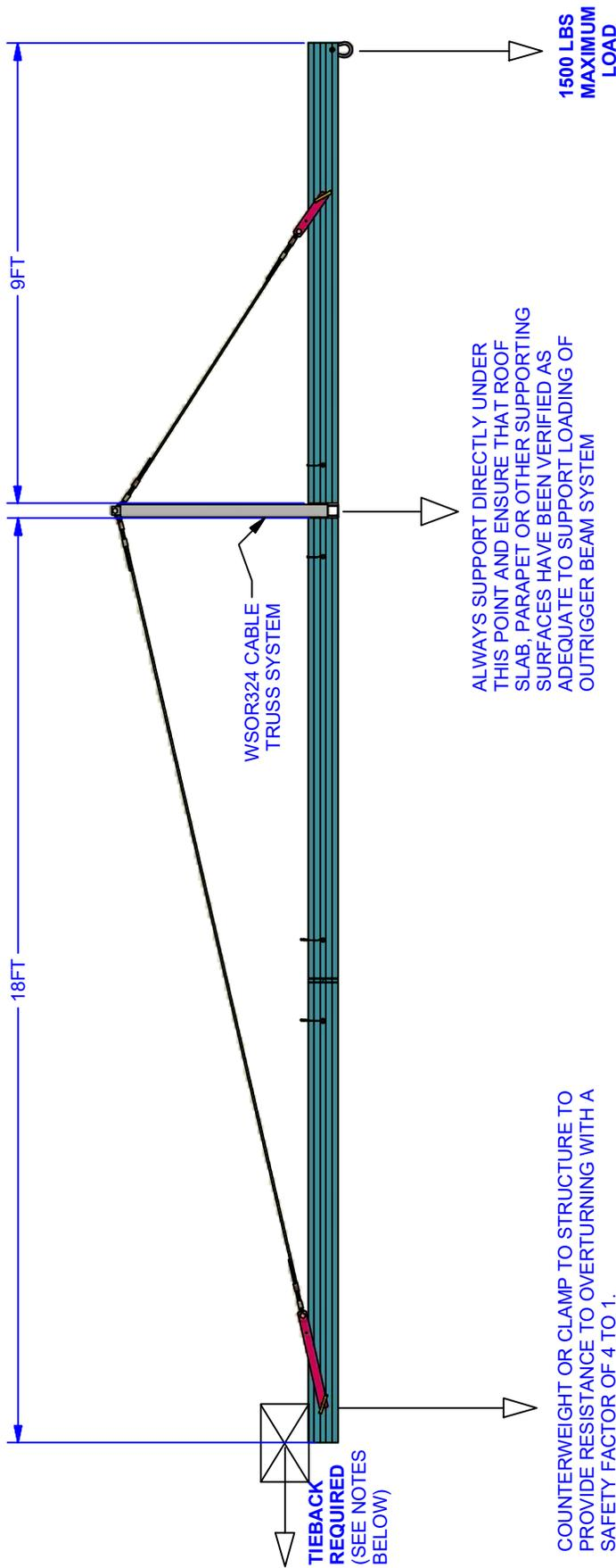
COUNTERWEIGHT OR CLAMP TO STRUCTURE TO PROVIDE RESISTANCE TO OVERTURNING WITH A SAFETY FACTOR OF 4 TO 1.
