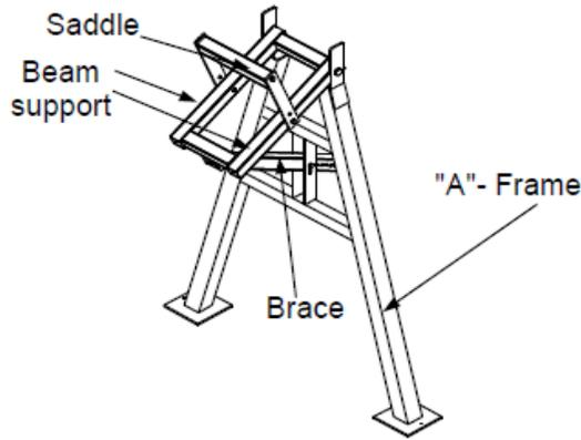
introduction of the 1500 Series outrigger beams, the saddle height has been increased. Winsafe beam stands can be refitted with the new Beam Stand Saddle (WSBS004) in order to be used with 1500 Series outrigger beams as well as standard Winsafe outrigger beams.
