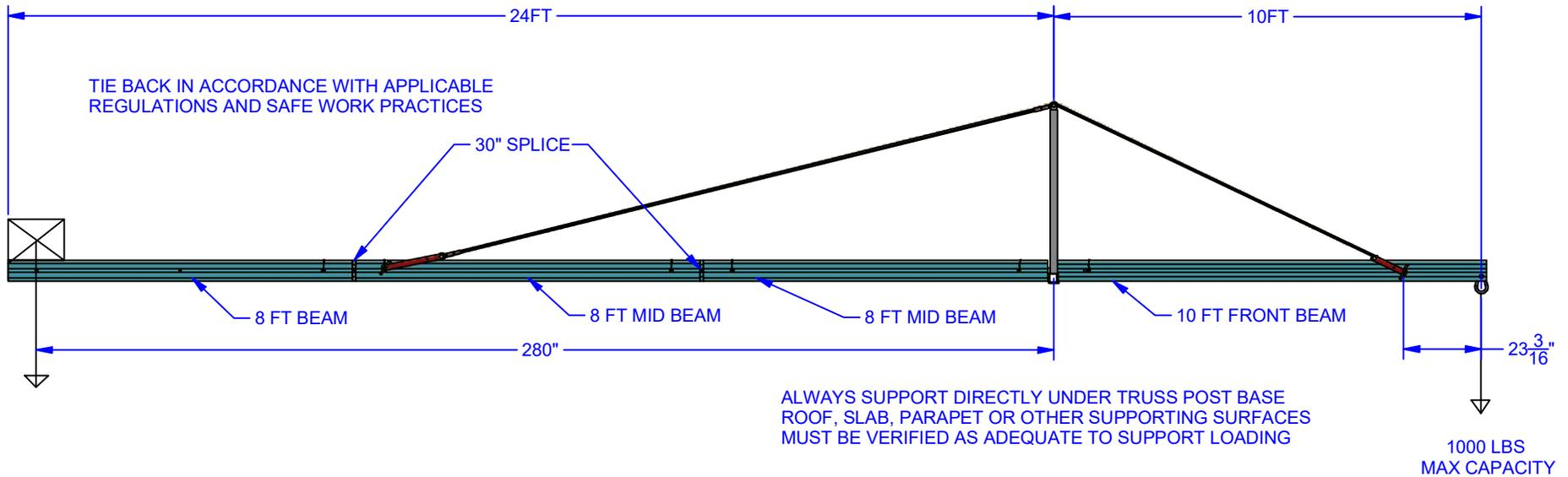
COUNTERWEIGHT OR CLAMP TO STRUCTURE TO PROVIDE RESISTANCE TO OVERTURNING WITH A SAFETY FACTOR OF 4 TO 1. REFER TO TABLE BELOW FOR REQUIREMENTS. USE COUNTERWEIGHT ADAPTERS TO SECURE ADDITIONAL WEIGHTS AS REQUIRED.
